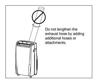
3. The exhaust hose supplied with the portable air conditioner has been specifically designed for this air conditioner. Do not lengthen the hose by adding additional hoses or attachments or replace it with any other hose.
